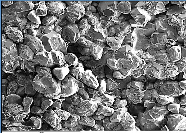
Scanning electron microscope (SEM) image of a Permo-Triassic sandstone showing the pore spaces between the grains; width of view 4.36 mm
