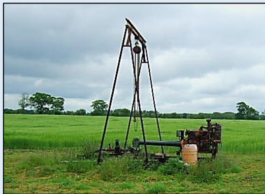
Diesel groundwater pump in use today, Staffordshire
