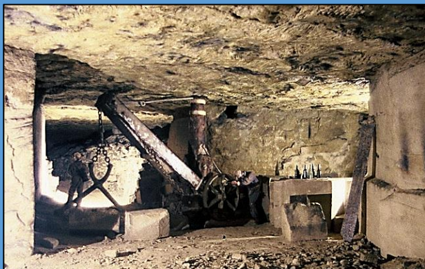
Box stone mine with an old block crane
