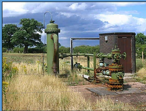
Brine pump near Warmingham, Cheshire; one of many pumps used for brine extraction
