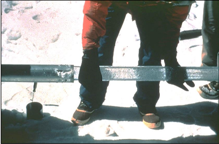
Figure 4.58. Extracting an ice core from a core tube taken from an ice borehole
