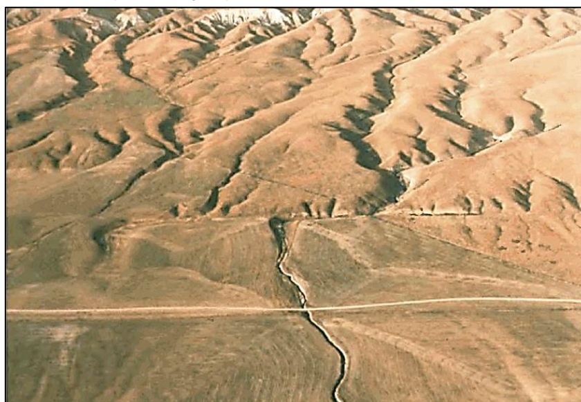
Figure 4.22. The San Andreas Fault in California, USA. The ground in the foreground has been faulted 130 metres to the left since the stream first cut its valley, offsetting it by this distance
