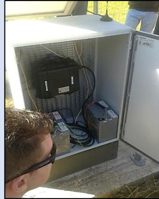
Recording equipment and back-up electricity supply for a Gulf of Corinth seismometer
