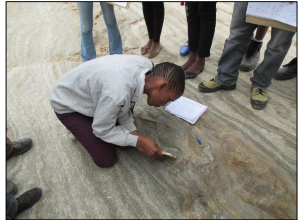
A student measuring dip and strike.
