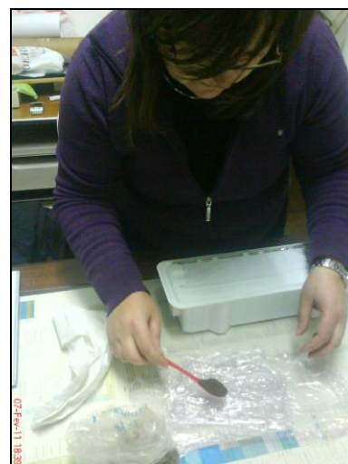
Preparation of samples for determining their magnetic susceptibility, Coimbra, Portugal, 2011 (Ana Rola).
