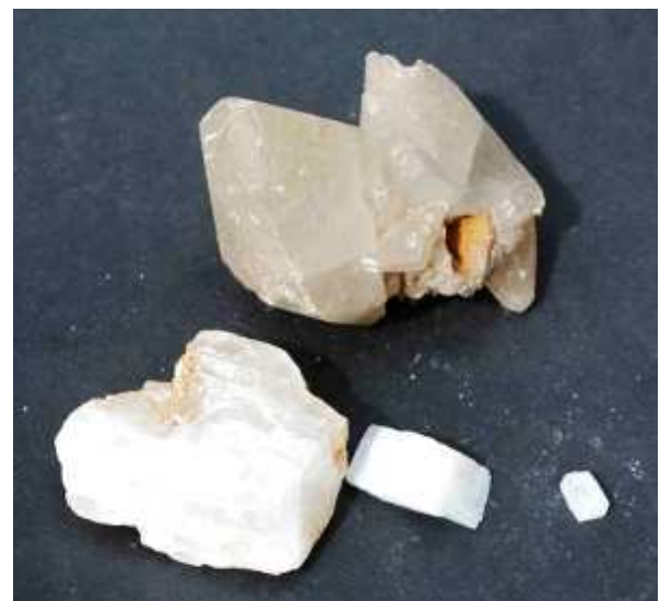
Cleavage: well-formed 'dog-tooth' crystals of calcite (top) with cleaved fragments of calcite (bottom)
