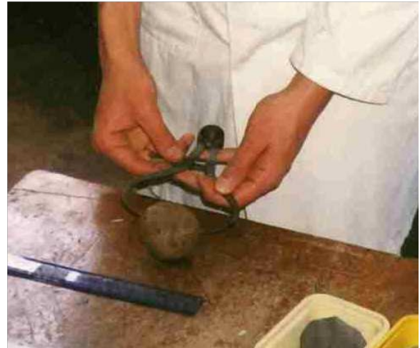
Measuring the diameter of the clay ball before dropping it, using callipers and a ruler (Photos: Peter Kennett )
