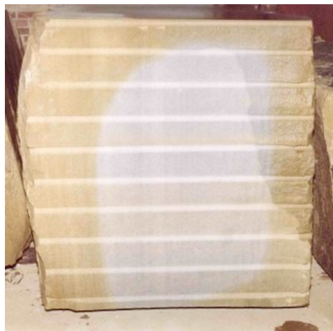
Drill holes in a block of sandstone, used in splitting the block from a larger mass, using 'plug and feathers' (The brown colour round the edges shows where weathering has oxidised the iron minerals in the rock). (Johnsons Wellfield, Huddersfield. Photo: Peter Kennett)
