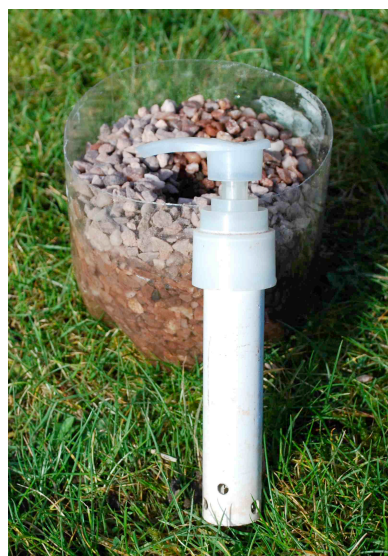
Showing a piece of perforated pipe around the pipe of the pump, to prevent clogging (see "Resources")
