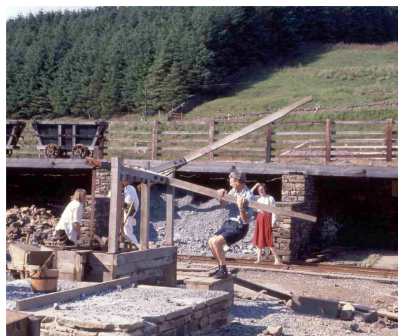
A full-size reconstruction of a jig on the ore-dressing floor at the Kilhope Mining Museum, County Durham
