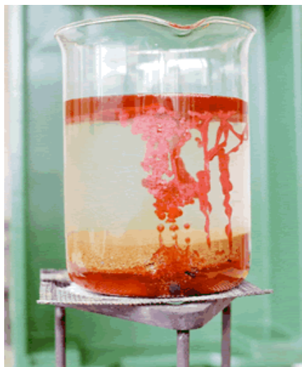
4 and 5. More feeder pipes develop and "intrusions" form as wax sets within the cold water
