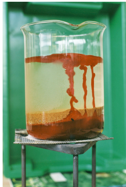
The wax volcano in action – in this example, a surface “lava flow” is fed by three feeder pipes, with “intrusions” building up near their bases – but all eruptions are different. (Photo: Peter Kennett)
