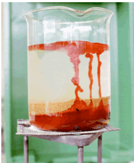
4 and 5. More feeder pipes develop and "intrusions" form as wax sets within the cold water
