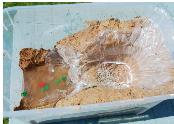
After the flood – the water has broken through the dam where the ice blocks have melted and washed away half a "village". (Photo: Peter Kennett)
