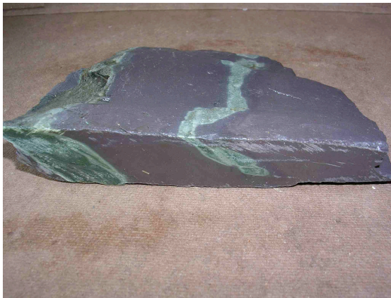
Slate showing colour banding from the bedding within the original mudstone. The slaty cleavage is parallel to the base of the specimen.
