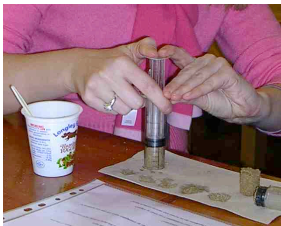
Making a 'rock' pellet in the lab using a sawn-off syringe
