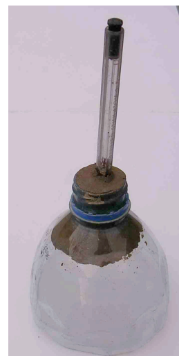
Home made funnel using the top of a bottle, a tube from a ball point pen and some clay (Photos: P. Kennett)
