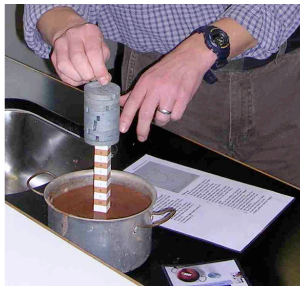
A teacher demonstrates how to measure pressure in the sand container (Photo: P. Kennett)
