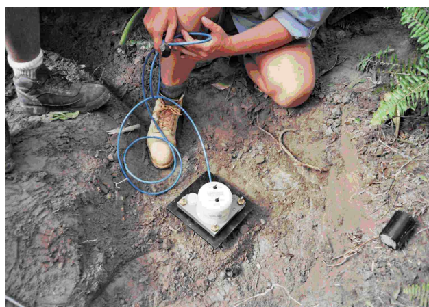
Tiltmeter in use on the volcanic island of Montserrat
